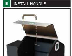
Flip hand around to the front and fasten to lid as shown here.
