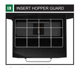
Open lid and install safety guard at base of hopper.
